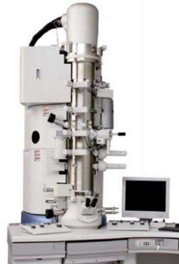
(b) A Hitachi Transmission electron microscope (HF3300) with an accelerating voltage of 330 kV, maximum magnification of 1.5 \times 10^6 \times and capable of resolving 0.13 nm. (Courtesy of Hitachi High-Technologies America Inc.)
